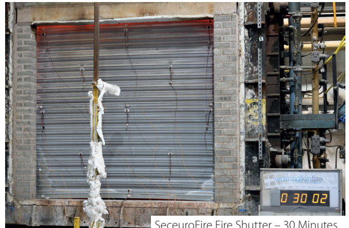
SeceuroFire Fire Shutter – 30 Minutes
