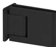
Agita Ultra black.edition Jet black, with hydraulic closing function and adjustable closing speed, max. door leaf weight 100 kg
